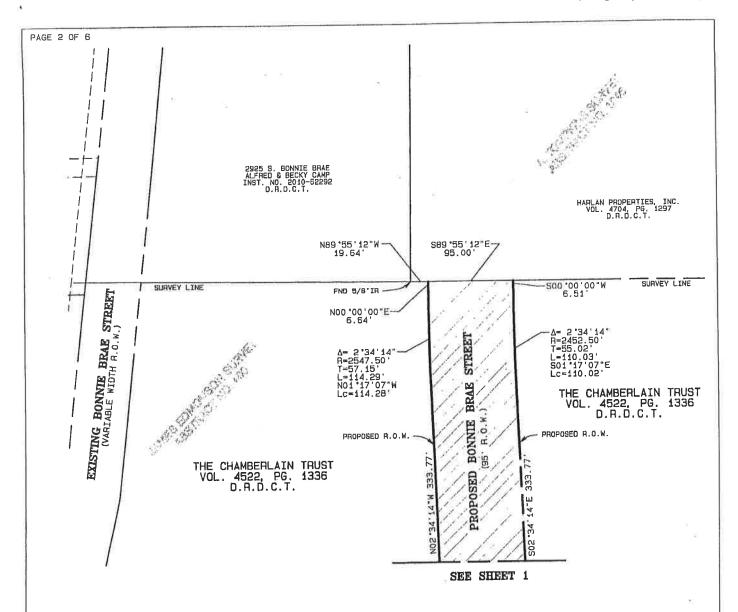
ALL PROPERTY CORNERS ARE SET 1/2"IR/ GAI CAP UNLESS OTHERWISE NOTED. BASIS OF BEARING IS NORTH AMERICAN DATUM OF 1983 (NAD-83) STATE PLANE COORDINATE SYSTEM, TEXAS NORTH CENTRAL.
